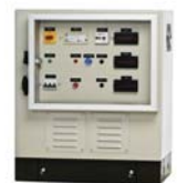
Tooling power supply unit
