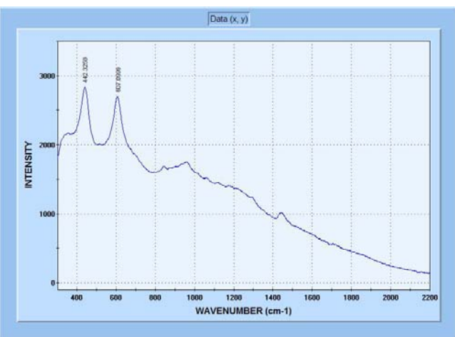
Fluorescence Spectrum of white epoxy paint chip
