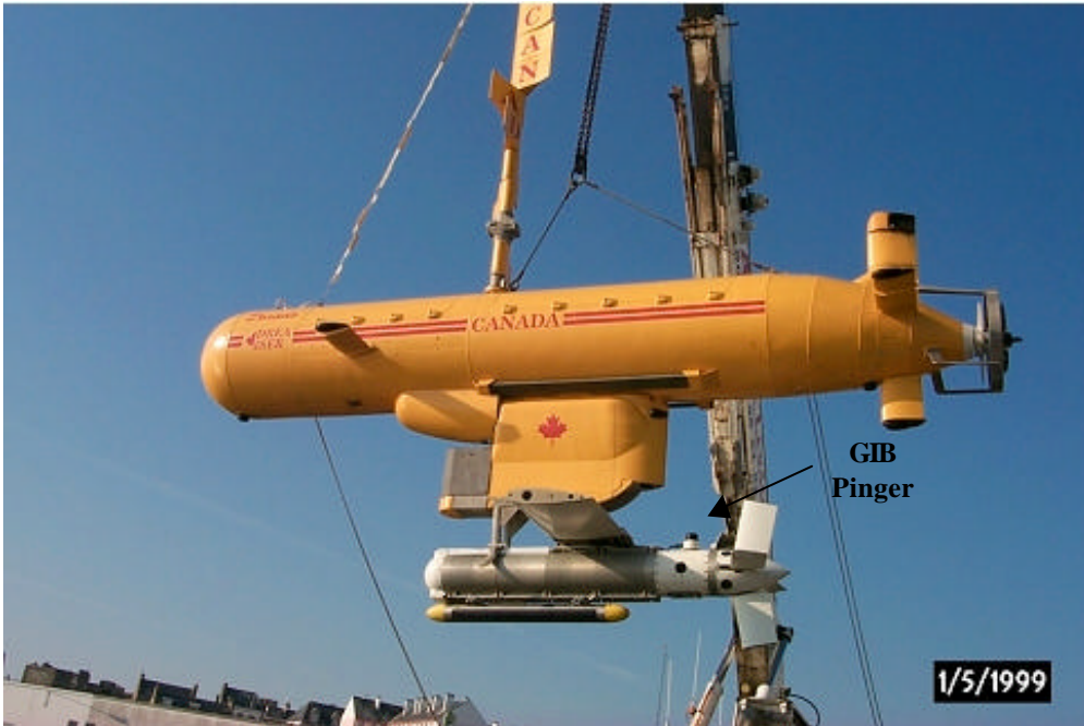
ISE semi-submersible MCM vehicle - GIB 10.5 kHz pinger
