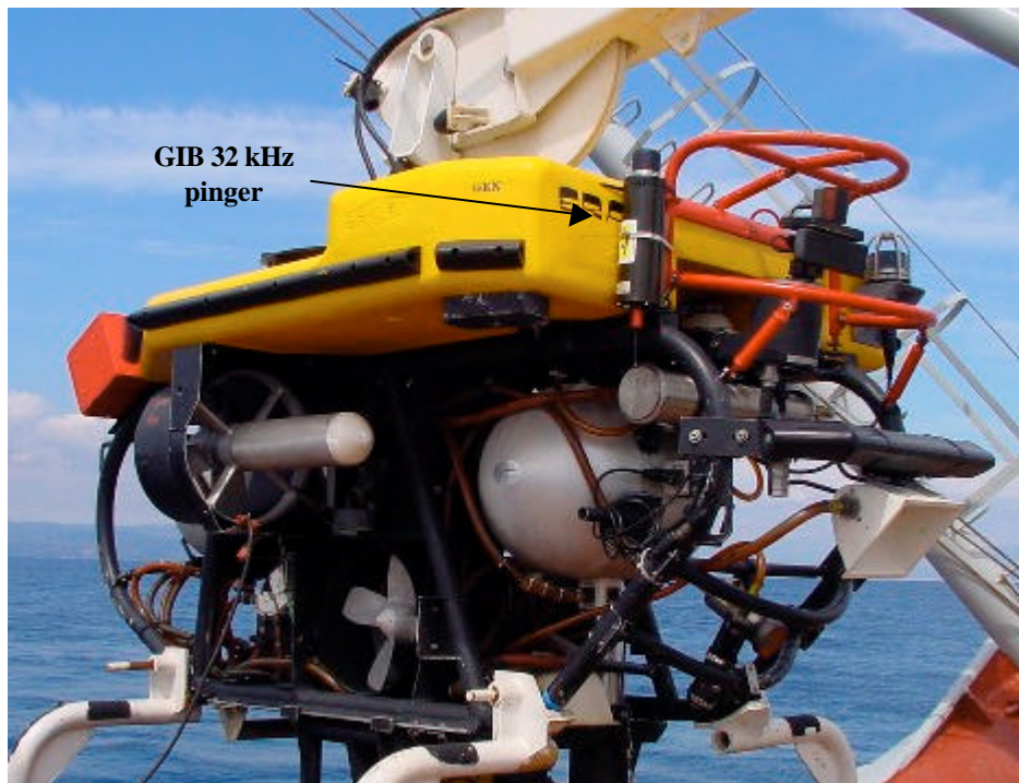
French Navy "ERATO" equipped with a GIB 32 kHz pinger
