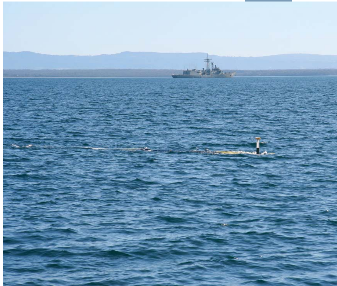
AUV 62 with the surveillance and communication mast in raised position.
