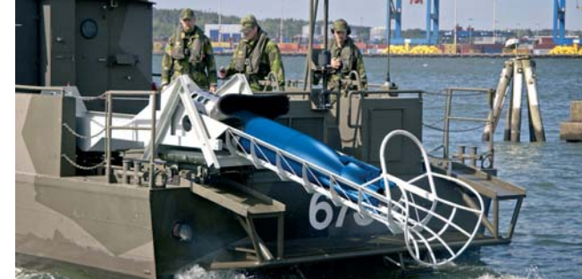
The docking device is reeled in, entering the chute, during recovery.
