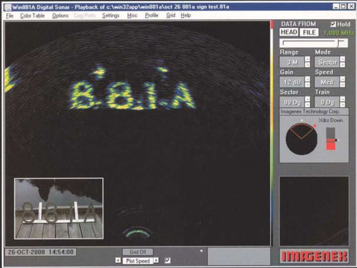
3M Sector Scan of Acoustic Sign at 1MHz. Inset: Photo of Acoustic Sign
